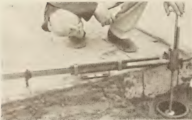
FIGURE 18.—DEVICE USED FOR MEASURING MOVEMENTS AT ENDS OF SLABS, AND BENCH MARK (LOWER RIGHT).
